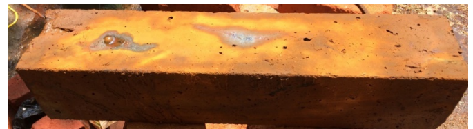
Figure 2 Corroded Prism Specimen
